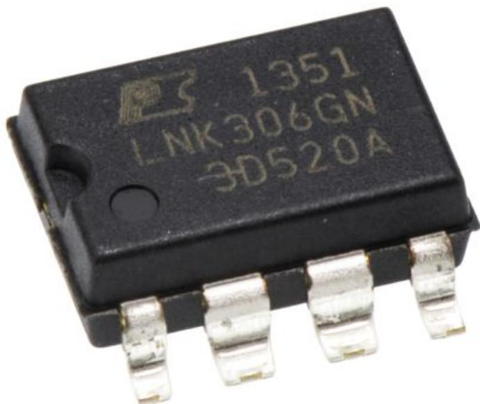
LNK306GN Switching Regulator, 12 V c.c., PDIP CMS 7 broches
