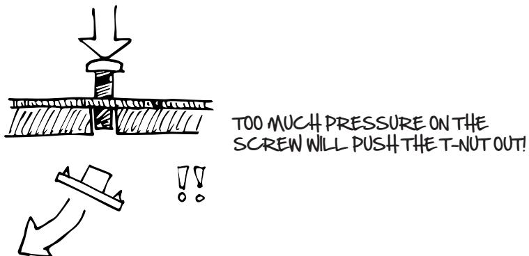
Tighten the screws slowly and carefully to make sure they do not cant - the nut can jam!
