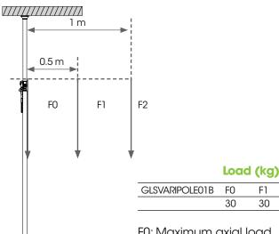
F0: Maximum axial load F1: Maximum load with 0.5 m arm
